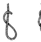
A Sheet Bend ties two ropes of unequal thickness together. It may be used in sailing to secure the main halyard to the clew outhaul when de rigging or it may be used to secure the forestay to the bow deck plate
